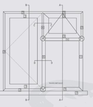
Face A - underbelly of ALL cills to be laminated as shown to ensure continuous colour when viewed from underneath.
